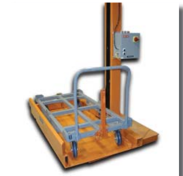
POST LIFT Ball and screw lift provides a 1/4" low profile to easily load the cart - capacity of 3000 lbs. Air or electric operated with push button controls mounted on post or free-standing pedestal. Ideal for narrow carts.
